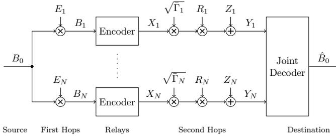
Fig. 1: Lossy-forward relaying system.
