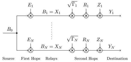
Fig. 2: Constrained end-to-end equivalent channel.
