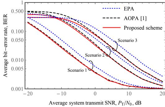
Fig. 3: Bit-error rates for two relays.
