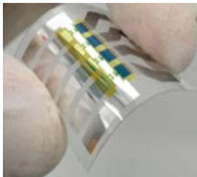
Fig. 2. photograph of a flexible PBT on a PET substrate
