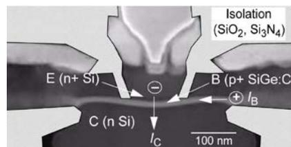
Fig. 7. TEM cross section of a 0.7THz SiGe:C npn HBT showing the relevant device regions and current flow directions.
