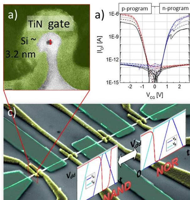
Fig. 5. Reconfigurable Si nanowire transistor. a) cross-section of device with omega gate and TiN electrode. b) Subthreshold transfer characteristics. c) 4T reconfigurable NAND-NOR cell with full output swing.
