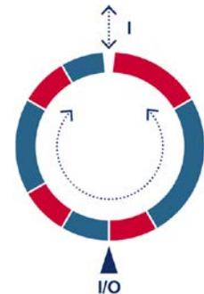
Fig. 5. Racetrack memory concept: A series of magnetic domain walls (boundaries between magnetic regions (red and blue) of opposite magnetization) are moved by current pulses (I) to an I/O device for reading and writing the domain walls.
