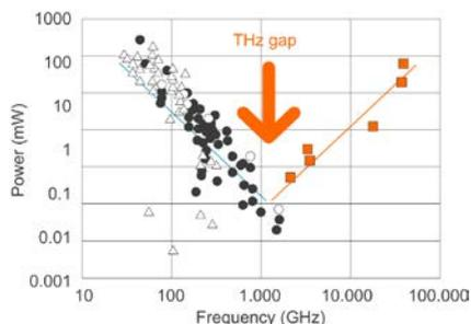
Fig. 6. The THz gap is generally defined by frequencies between 300GHz to 30THz (i.e. by wave lengths between 1mm and 10 $\mu$ m). (image: [25])
