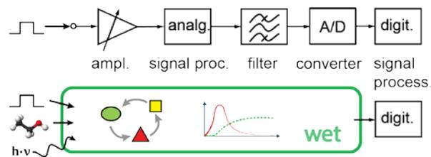
Fig. 9. The biomolecular near-sensor processor operates next to biomolecular sensors and simultaneously replaces sequential processing by standard engineered routines such as amplifier, analog signal processing, filter and A/D converter. It directly provides robust decision signals in response to multichannel inputs, even at few-molecule resolution
