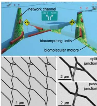
Fig. 8. Schematic of a programmable molecular-motor based computer
