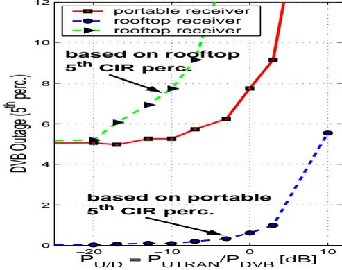
Figure 2: DVB-T outage versus power ratio
