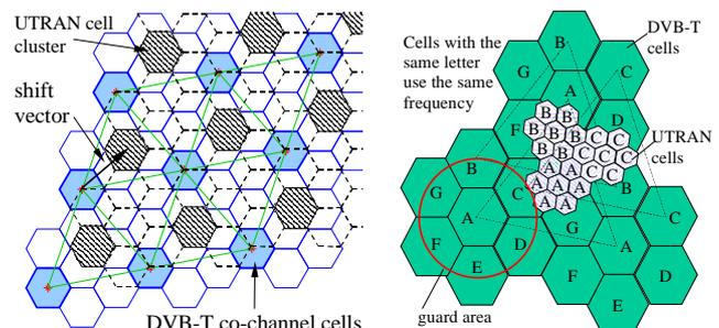
Figure 1: Superimposed layouts of DVB-T cells and UTRAN cell clusters;
