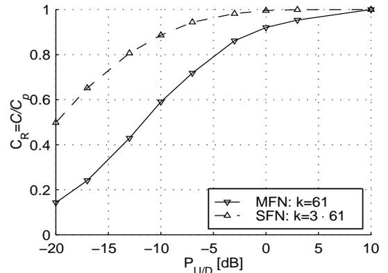
Figure 3: Relative capacity for MFN and SFN; reuse 7
